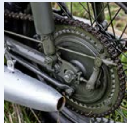
ABOVE: Bolt-over 56-tooth rear sprocket lowers gearing for off-road action. The standard sprocket is 46-tooth
