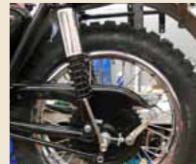
Unusual shocks on McQueen's machine went without the lower covers and featured black springs
