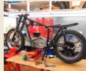
Frame went largely unmodified. Primary drive is by chain – none of your fancy belt conversions here
