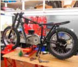
Frame went largely unmodified. Primary drive is by chain – none of your fancy belt conversions here
