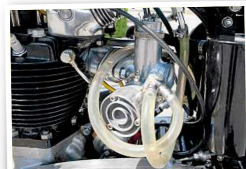
Twin carbs are mounted on a Webco manifold.
