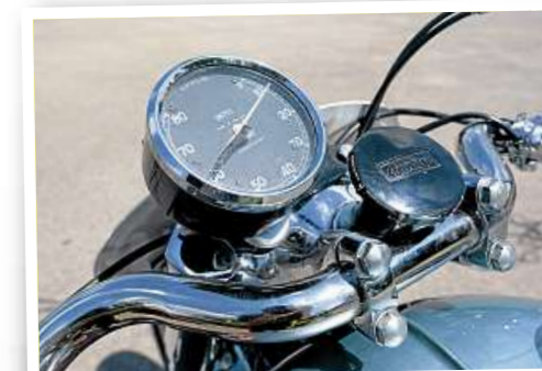
Rev counter mounting bracket is to the Triumph GP pattern.
